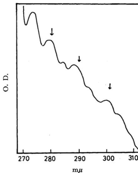
Fig. 2. The spectra of cyclohexane-1,4-dione in the E.P.A. solution at 77°K.
